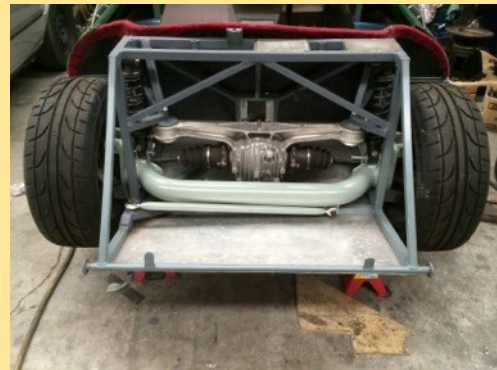
Old meets new- De Dion Rear end, grafted to a LSD MX5 IRS Note the extra bracing for the Rollcage
