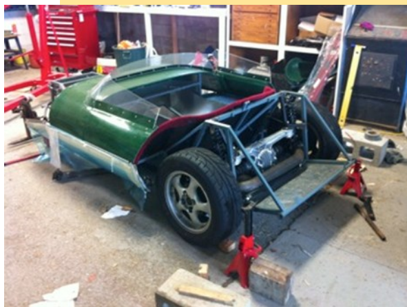
Old meets new- De Dion Rear end, grafted to a LSD MX5 IRS Note the extra bracing for the Rollcage
