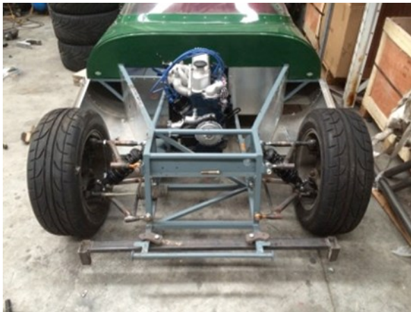
First fitting of the Crossflow and 5 speed type 9 gearbox
